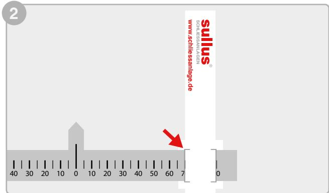
The part printed with the length scale is pushed through the pre-cut slots of the legs.
