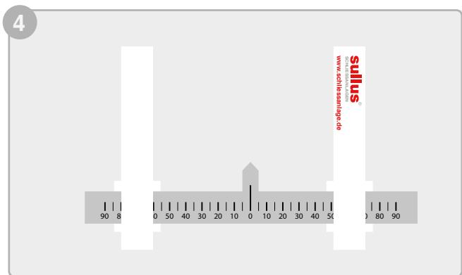
Please check the length indication on the scale with a ruler. When mounted correctly, the readable dimension is correct.
