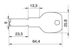
The authorization check on Akura 44 cylinders occurs in several levels simultaneously, namely through the combination of a variable length profile, 6 active and up to 10 passive scanning pins, which also extend the calculation capacities. Optional magnetic copy protection protects critical access points, if required and makes it difficult to copy keys or manipulate with the cylinder.
